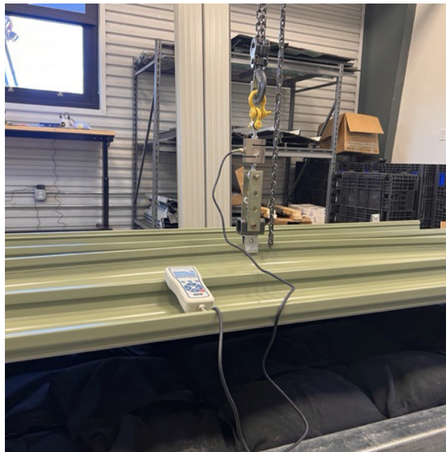
Fig 5: S-5-HR clamp mounted mid-span holding load
