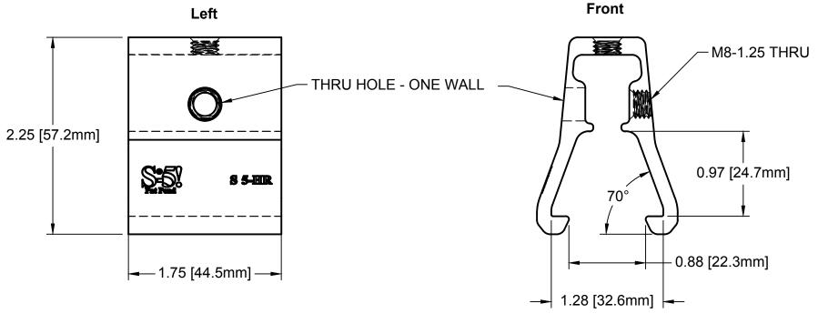
MATERIAL: METAL ROOF INNOVATIONS, LTD. 6000 Series Al 8750 WALKER RD EST ASSEMBLY WT: COLORADO SPRINGS, CO 80908 0.18 LB 719-495-0518 719-495-0045 (FAX) HARDWARE: 30mm M8 Bolt - T30 DRIVE S-5-H [CCD] DRAWING NO. HRPV-A-0-A DRAWN BY SB 03/15/2023 HRPV-A-0-A (S-5-H) [CCD] S-5!® PRODUCTS ARE PROTECTED BY MULTIPLE U.S. AND FOREIGN PATENTS. VISIT OUR WEBSITE AT WWW.S-5.COM FOR COMPLETE INFORMATION ON PATENTS AND TRADEMARKS
