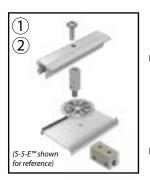
Assemble the HUR prior to installing on the roof. Place the baseplate then the PV disk atop the clamp and thread the male portion of the standoff through the disk and baseplate into the clamp. Assemble the baseplate so the lip facing upward is the lip located closest to the module flange. First try the side with the smaller lip spacing. If there is interference with the flange, then flip to the larger spacing (Figure 1a).
