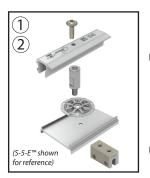
Assemble the PVKIT HUR prior to installing on the roof. Place the baseplate then the PV disk atop the clamp and thread the male portion of the standoff through the disk and baseplate into the clamp. Assemble the baseplate so the lip facing upward is the lip located closest to the module flange. First try the side with the smaller lip spacing. If there is interference with the flange, then flip to the larger spacing (Figure 1a).
