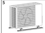
(Split System/HVAC unit mounted with (4) Levelers on one side and and (2) damper pads).
