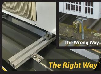
Securely attaches rooftop utilities to exposed-fastened roof while still allowing free flow of rainwater under the system. All you need is the GRIPPERFIX Strut, S-5! self-piercing fasteners and EF Tabs. M8 bolts in different lengths are available to use with the optional damper pad(s). The GRIPPERFIX Leveler allows for the leveling of rooftop utilities up to 5 degrees when needed.
